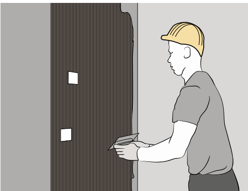
Spread adhesive on plaster
